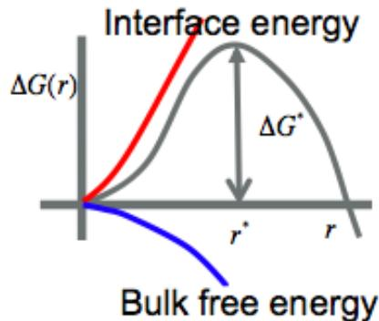
Two terms contribute to this. A volume term (blue line),  $\sim r^3$ , which takes into account the gain in free energy associated to the formation of the crystal, and a surface term that is connected to the work required to create the crystal-liquid interface (red line),  $\sim r^2$ . The balance of these contribution results in a maximum, this is the activation free energy for the formation of the critical nucleus of radius  $r^*$ .
