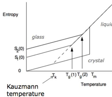
The Kauzmann temperature corresponds to the intersect of the entropy of the supercooled liquid with the entropy curve of the crystalline solid. Because the entropy of the glass cannot be smaller than that of the crystal the Kauzmann T marks a lower limit in the experimental glass transition temperature.
