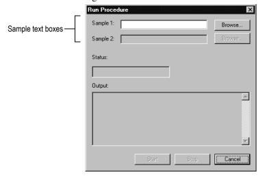
The dialog box features a **Sample n** text box, where **n** is the sample number, for each of the chemical samples used. For example, a procedure with two input arguments has a text box for Sample 1 and a text box for Sample 2.
