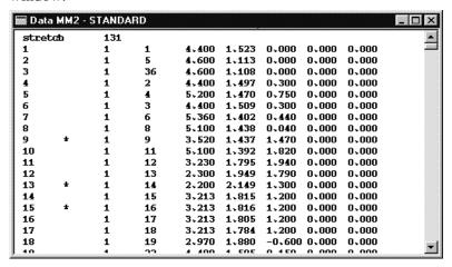
Edit the figures in the window to change the parameter data set. If any unsaved changes have been made to the data set, the title bar displays an asterisk symbol (\*).
