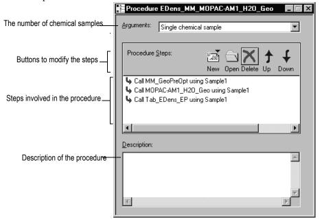
Use the five buttons in the Procedure Steps section to modify the existing procedure. In addition, you can use the menu options in the Procedure window to modify the procedure.
