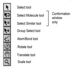
You can rotate, translate, and zoom in to the map and conformation window using the tools, and also select items with the three selection tools in the conformation window. Using the Select tool in the graph window changes the position of the spherical marker in the graph.
