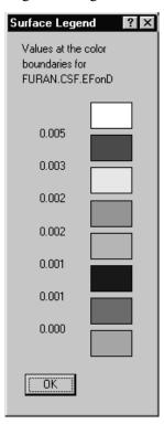
The Surface Legend dialog box displays the threshold value of transition from one surface color to another for the selected surface. The colors displayed depend on the current colors assigned to each of the color indexes listed in the following CAChe color tables.
