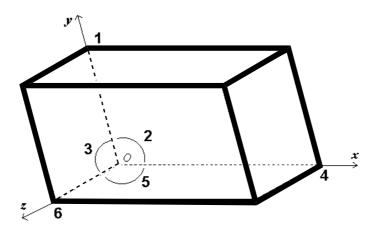
(iii) With reference to the picture of a unit cell shown below, give the indices for the two planes 1 and 2.
