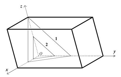
(iv) The figure shows a 2-fold rotation axis along z with a perpendicular xy mirror plane at z = 0. What are the general coordinates associated with the four positions (1), (2), (3) and (4). What additional symmetry element is generated by the combination of the 2-fold rotation and the perpendicular mirror plane, and where is it?
