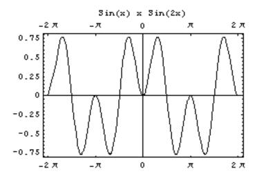
The symmetry of the plot makes it clear that an integral of this function over any period of  $2\pi$  will yield 0.
