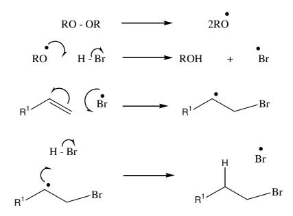
The overall result is an anti-Markovnikov addition of HBr i.e. to give the opposite regioisomer from that formed in electrophilic addition of HBr. However, the reason for the regiochemistry is the same as that in the electrophilic addition, namely, that the most stable intermediate (radical in this case) is formed and the reversal of regiochemistry is purely because Br adds first instead of H.
