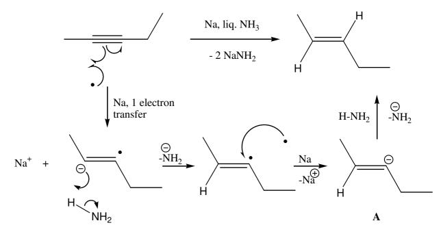
The carbanion **A** can adopt either the cis or trans configuration but prefers the latter because in that configuration there is less steric hindrance between the two alkyl groups on the double bond:
